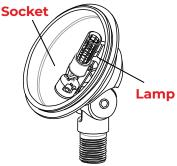
Insert the lamp with the correct wattage and type marked on the luminaire label.
