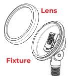
Thread the lens back onto the luminaire and hand tighten until snug.
