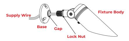
Place the supply wire through the base and thread the base onto the fixture body. Make sure the gap on the base and the fixture body are in the same direction. Tighten the lock nut against the base.
