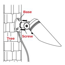
Pull the supply wire through the gap on the base. Attach the base onto the tree by securing with the screws. Tighten with a screwdriver.
