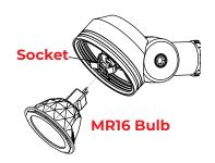
Insert the MR16 bulb with the correct wattage and type marked on the fixture label and secure into place.
