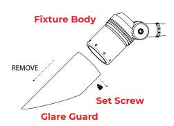
Loosen the set screw and remove the glare guard from the fixture body.
