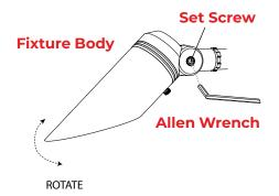
By using an Allen wrench, loosen the set screw on the knuckle and adjust the fixture body to the desired direction. Once the desired direction is achieved, tighten the set screw to secure.
