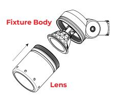
Place the lens back onto the fixture body and rotate it until it is secured properly.
