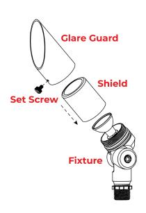
Attach the shield back onto the fixture. Place the glare guard over the shield and secure with the set screw. Tighten until snug.
