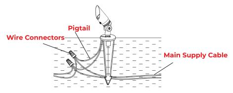
Strip both leads from the luminaire pigtail. Using two wire connectors (sold separately), connect the leads from the luminaire to the main supply cable leads.
