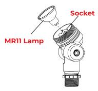
Insert the lamp with the correct wattage and type marked on the fixture label.
