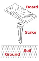
Determine the desired location for mounting the fixture. Hammer the stake into the ground until flange of stake is flush to grade. To avoid damage to the stake, place a board on top of the stake while hammering.
