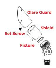
Loosen the set screw and remove the glare guard from the shield. Loosen the shield and remove it from the fixture.
