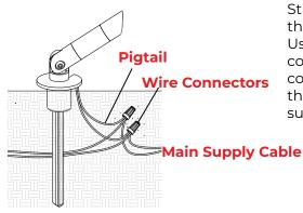
Strip both the leads from the luminaire pigtail. Using two UL listed wire connectors (sold separately), connect the leads from the luminaire to the main supply cable leads.
