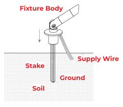
Insert the stake into the soil until flange of stake is flush to the ground.
