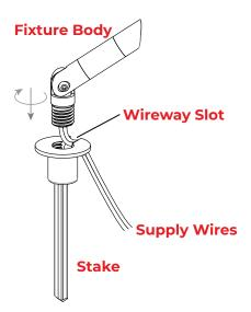
Pass the supply wire of the fixture body through the wireway slot on the stake. Thread the fixture body onto the stake.
