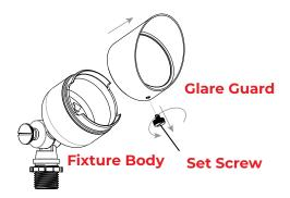
Loosen the set screw and remove the glare guard from the fixture body.
