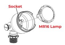
Insert MR16 lamp with correct wattage and type marked on fixture label.
