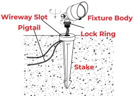
Clear away an area in the ground at the wireway slot on top of the stake. Lay the luminaire pigtail into the wireway slot and screw the fixture body on to the stake. Tighten the lock ring against the stake and hand tighten until snug.
