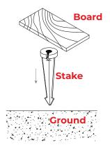
Determine the desired location for mounting the fixture. Hammer the stake into the ground until flange of stake is flush to grade. To avoid damage to the stake, place a board on top of the stake while hammering.
