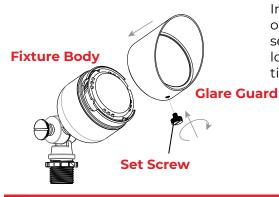
Install the glare guard back onto the fixture body and secure with previously loosened set screw. Hand tighten until snug.
