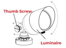
Loosen the knuckle screw at the joint. Rotate the luminaire to your desired direction. Tighten the knuckle screw once your desired direction is achieved.
