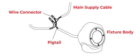
Place fixture body on your desired location. Strip both leads from luminaire pigtail. Using two UL listed wire connectors (sold separately), connect the leads from the fixture body to main supply cable leads. Make this connection at least 10 feet outside of the water.
