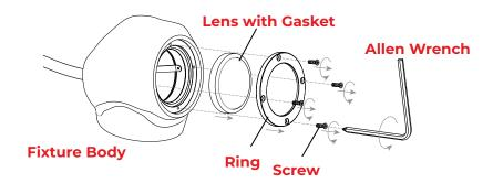
By using the screwdriver end of the Allen wrench, loosen four screws and remove them from the fixture body. Remove the ring and the lens with gasket.
