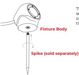
Thread the spike (sold separately) into the bottom of the fixture body. Hand tighten until snug.
