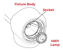
Insert MRII lamp with correct wattage and type marked on fixture label.
