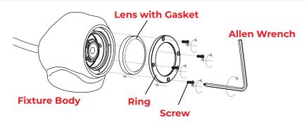
Place the lens with gasket and the ring back onto the fixture body. By using the screwdriver end of the Allen wrench, thread previously removed four screws back onto the fixture body. Hand tighten until snug.
