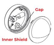
Push the lens assembly back onto the base aligned with the gaps on the base. Push hard (moisture proof fixture requires force to get air out). Once the lens assembly is flush with the base, rotate the lens assembly until it stops and locks into place.
