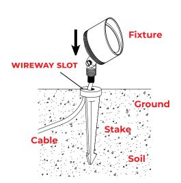
Clear away an area in the ground at the wireway slot on the top of the stake. Place the fixture wire into the wireway slot and thread the fixture onto the stake. Hand tighten until snug.
