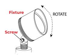
Loosen the knuckle and adjust the fixture to the desired orientation. Tighten the knuckle after you find the desired orientation.
