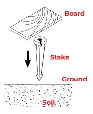
Determine the desired location for mounting the stake. Hammer the stake into the ground until flange of stake is flush to grade. To avoid damage to the stake, place a board on top of the stake while hammering.
