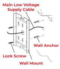
Place the wall mount at the desired location and mark two points on the wall surface for the wall anchors. Remove the wall mount and drill the proper holes on the wall.
