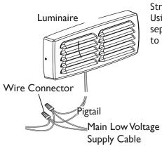
Strip two leads from luminaire pigtail. Using two wire connectors, sold separately, connect leads from luminaire to main low voltage supply cable leads.
