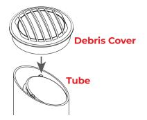
Attach the debris cover onto the top end of the tube if necessary.
