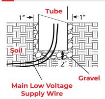
Dig a 6.5" diameter, 8" deep hole in the ground. Run the main low voltage supply wires to the hole.
