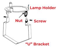
Attach the lamp holder onto the "U" bracket by lining up the holes, then pass the screws through the holes and secure with the provided nuts.
