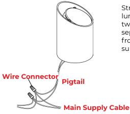
Strip both leads from the luminaire pigtail. Using two wire connectors (sold separately), connect the leads from the luminaire to the main supply cable leads.
