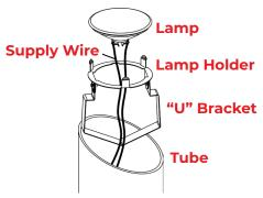
Use the PAR36 lamp with the correct wattage and type marked on the fixture label.
