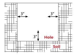
Prepare a hole in the ground. Make sure there are approximately 3" spaces surrounding the fixture for pea gravel or sand.
