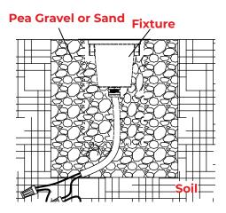
Install the fixture in the hole and fill the hole with pea gravel or sand.
