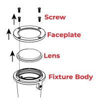
Use a screwdriver to loosen the screws on the faceplate and remove the lens from the fixture body.
