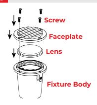
Place the lens and the faceplate back onto the fixture body and secure the removed screws in a star pattern using a screwdriver. Tighten until snug.
