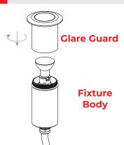
Thread the glare guard back onto the fixture body and hand tighten until snug.
