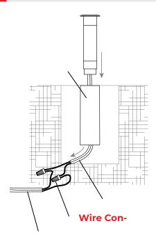
Pass the fixture wire through the PVC tube. Place the fixture body into the PVC tube.
