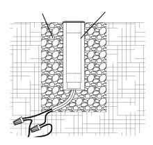
Install the PVC tube with fixture in the hole and fill hole with pea gravel or sand.
