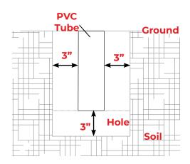
Dig a hole in the ground with approximately 3" of space surrounding the PVC tube for pea gravel or sand.
