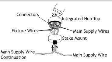
Insert the main supply wire continuation (if needed) and the main supply wire up through the bottom of the stake mount and strip the ends of both sets of supply wires.
