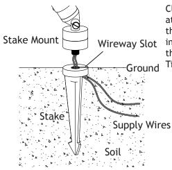
Clear away an area in the ground at the wireway slot on top of the stake. Lay the supply wires into the wireway slot and screw the stake mount on to the stake. Tighten until snug.
