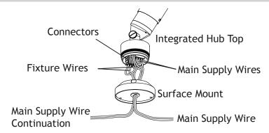
Insert the main supply wire continuation (if needed) and the main supply wire up through the bottom of the surface mount and strip the ends of both sets of supply wires.
