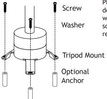
Place the tripod mount onto the desired location and secure it with the screws. Tighten with a screwdriver. Nylon spacers are required when installing on trees.
