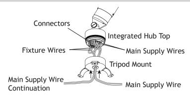
Insert the main supply wire continuation (if needed) and the main supply wire up through the bottom of the tripod mount and strip the ends of both sets of supply wires.
