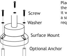
Place the surface mount onto the desired location and secure it with the screws. Tighten with a screwdriver. Nylon spacers are required when installing on trees.
