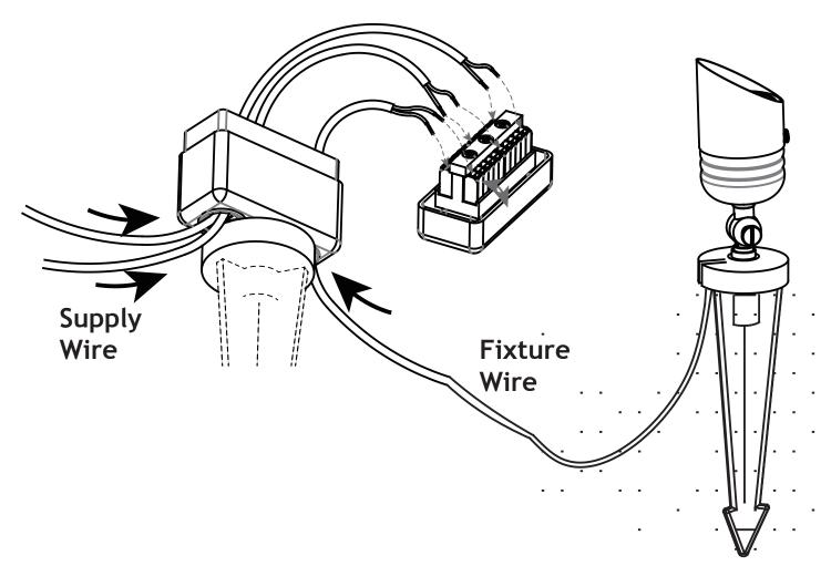
C. Run the fixture wire to the hub and insert the wire through the rubber grommets on the bottom of the hub. Then, flip one of the terminal levers open, insert one end of the stripped fixture wire, and flip the lever closed to make your connection. Last, flip the lever open that is directly opposite from the first fixture wire connection, on the other side of the terminal block, and insert the other end of the fixture wire and flip the lever closed to make the connection.
