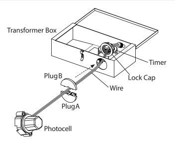
Open the transformer door by releasing the latch on its side. Run the wires from the photocell through the hole on the side of the transformer box. Clamp the photocell wires by using both of the plugs. Insert plugs A and B simultaneously into the hole on the side of the transformer box, then secure it with the lock cap and hand tighten until snug. Connect the plug of the wire into the timer.
