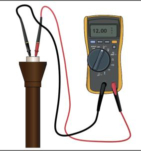
If needed, you can adjust the fixture voltage by using a higher voltage at the transformer terminal.
