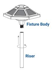
Thread the riser onto the fixture and hand tighten until snug.
