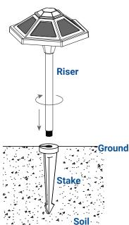
Thread the riser on to the stake and hand tighten until snug.
