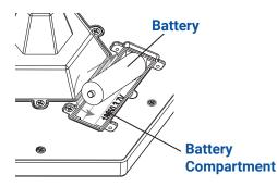
Insert the battery into the battery Compartment.
