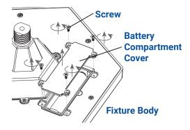
Using a screwdriver, remove the battery compartment cover from the fixture body.
