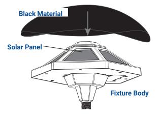
Cover solar panels completely by using black materials. The fixture will light up when the solar panel is covered and turn back off when it is uncovered.
