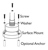
Place the surface mount onto the desired location and secure it with the screws. Tighten with a screwdriver.
