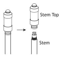
Twist the stem top counterclockwise and remove it from the stem.
