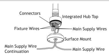
Insert the main supply wire continuation (if needed) and the main supply wire up through the bottom of the surface mount and strip the ends of both sets of supply wires.
