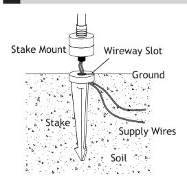
Clear away an area in the ground at the wireway slot on top of the stake. Lay the supply wires into the wireway slot and screw the stake mount on to the stake. Tighten until snug.
