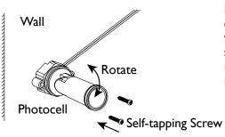
Place the photocell at your desired location and secure with self-tapping screws. Make sure the photocell is in the right directioin so that it can be rotated up.
