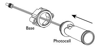
Pass the cord through the base and thread the photocell onto the base. Hand tighten until snug.
