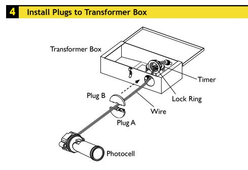
Open the transformer door by releasing the latch on its side. Run the wires from the photocell through the hole on the side of the transformer box. Clamp the photocell wires by using both of the plugs. Insert plugs A and B simultaneously into the hole on the side of the transformer box, then secure it with the lock cap and hand tighten until snug. Connect the plug of the wire into the timer.
