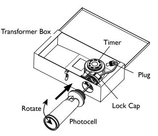
Open the transformer door by releasing the latch on its side. Run the wires from the photocell through the hole on the side of the transformer box. Place the photocell onto the hole on the side of the transformer box and make sure the photocell is in the right direction so that it can be rotated up. Secure it with the lock cap and hand tighten until snug. Connect the plug of the wire into the timer.
