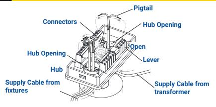
Put the supply cables from the transformer and the fixtures through the openings on the bottom of the hub. Each opening can accept four cables. Strip each end of supply cable pigtail. Open the lever on the terminal block connector. Insert one side of the pigtail into the connector on the terminal block and push the lever down to secure the connection. Insert the other side of the pigtail into the opposite connector and push the lever down to secure the connector.
