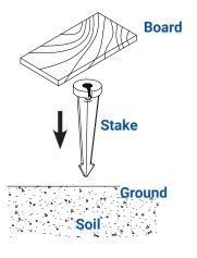
Determine the desired location for mounting the stake. Hammer the stake into the ground until flange of stake is flush to grade. To avoid damage to the stake, place a board on top of the stake while hammering.
