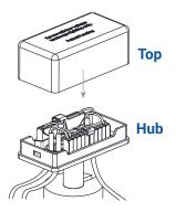
After all wires are connected, carefully pull the extra wire out of the bottom openings of the hub. Then, place the cover back onto the hub.
