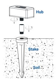
Thread the riser and the hub onto the stake. Hand tighten until snug.
