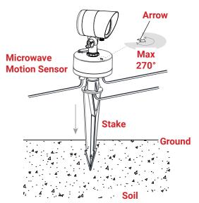
Aim the arrow on the microwave motion sensor to the desired detective area. The maximum detective range is 270°.
