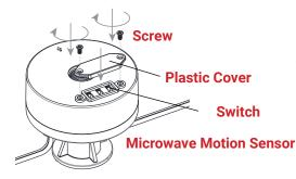
Place the plastic cover back on top of the switches and secure with the previously removed screws.
