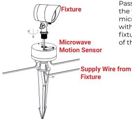
Pass the supply wire from the fixture through the microwave motion sensor with the stake. Thread the fixture onto the top center of the sensor.
