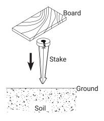
Determine the desired location for mounting the hub. Hammer the stake into the ground until flange of stake is flush to grade. To avoid damage to the stake, place a board on top of the stake while hammering.
