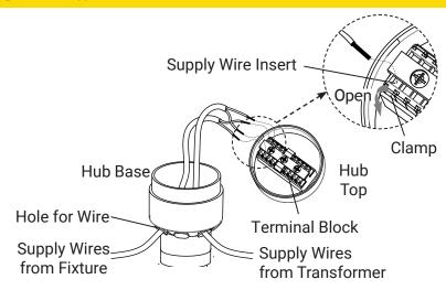
Pass the supply wires from the transformer through one of the holes underneath the hub base. Strip both leads of the supply wire from the transformer. Open the clamp on the connector that you are going to insert the wire in, insert one side of the supply wire into the connector on the terminal block and close the clamp. Then insert the other side of the wire into the opposite terminal block.
