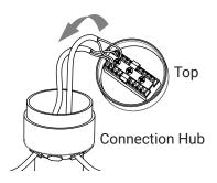
After the wires are well connected, place the top back onto the connection hub. Leave any access wire inside of the hub in case you need to adjust the placement of the fixtures.
