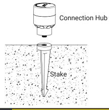
Hand tighten the connection hub to the stake until snug.
