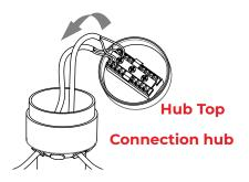
After the wires are well connected, place the top back onto the connection hub. Leave any access wire inside of the hub in case you need to adjust the placement of the fixtures.
