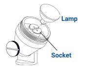
Insert the lamp (sold separately), with the correct wattage and type marked on the luminaire label.
