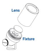
Thread the lens onto the luminaire and hand tighten until snug.
