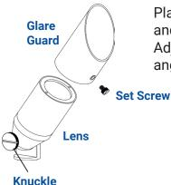
Place the glare guard over the lens and secure with the set screw. Adjust the luminaire to the desired angle by using the knuckle.
