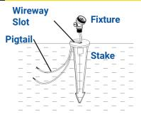
Clear away area in the ground at the wireway slot on top of the stake. Lay the luminaire pigtail into the wireway slot and tighten fixture on to stake.
