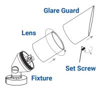
Unlock the set screw and remove the glare guard from the lens. Unscrew the lens to remove it from fixture.
