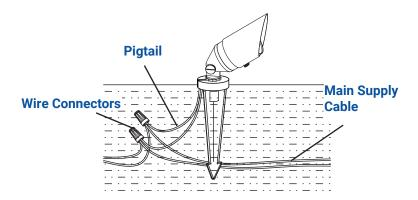
Strip both the leads from the luminaire pigtail. Using two UL listed wire connectors (sold separately), connect the leads from the luminaire to the main supply cable leads.
