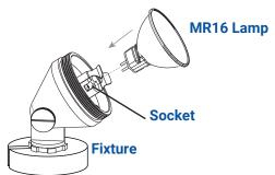
Insert MR16 bulb with the correct wattage and type marked on the fixture label and secure into place.
