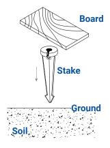
Determine the desired location for mounting the stake mount. Hammer the stake into the ground until flange of stake is flush to grade. To avoid damage to the stake, place a board on top of the stake while hammering.
