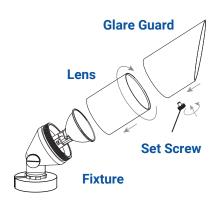
Thread the lens back onto the fixture and hand tighten. Place the glare guard back onto the lens and secure with previously removed set screw.
