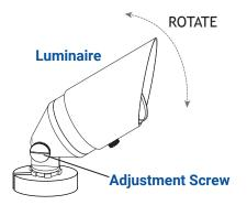
Loosen the adjustment screw at the joint and adjust the luminaire to the desired direction. Once the desired direction is achieved, tighten the adjustment screw.
