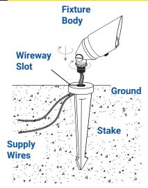
Clear away an area in the ground at the wireway slot on top of the stake. Lay the supply wires into the wireway slot and attach the fixture on to the stake. Tighten until snug.
