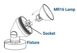
Insert MR16 bulb with the correct wattage and type marked on the fixture label and secure into place.
