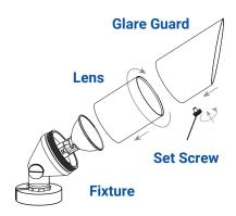
Thread the lens back onto the fixture and hand tighten. Place the glare guard back onto the lens and secure with previously removed set screw.
