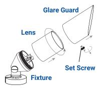
Unlock the set screw and remove the glare guard from the lens. Unscrew the lens to remove it from fixture.
