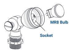
Insert MR8 bulb with correct wattage and type marked on fixture label.
