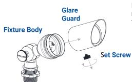
Loosen the set screw and remove the glare guard from the fixture body.
