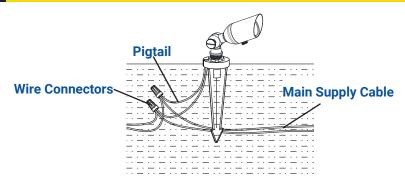
Strip both the leads from the luminaire pigtail. Using two UL listed wire connectors (sold separately), connect the leads from the luminaire to the main supply cable leads.
