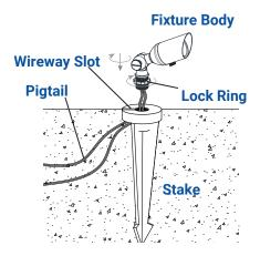
Clear away an area in the ground at the wireway slot on top of the stake. Lay the luminaire pigtail into the wireway slot and screw the lamp body on to the stake. Tighten the lock ring against the stake and hand tighten until snug.
