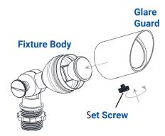
Place the glare guard back onto the fixture body and secure with previously removed set screw.
