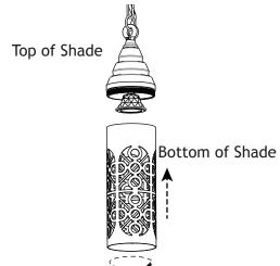
Thread the top of the shade back onto the bottom of the shade.
