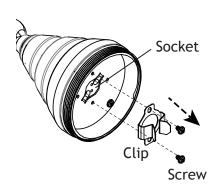
Remove the clip from the socket by removing the screws.
