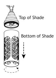
Remove the top of the shade from the bottom of the shade to expose the socket.
