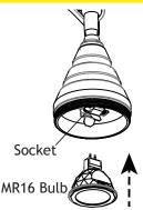
Insert the MR16 bulb with the correct wattage and type marked on the fixture label.
