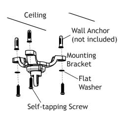
Attach the mounting bracket onto the desired ceiling surface. Secure with the flat washers and self-tapping screws.
