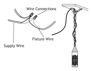
Strip both leads from the luminaire pigtail. Connect the leads from the luminaire supply cable to the transformer (sold separately).
