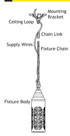
Adjust the fixture chain to the desired length by removing the links if needed. (Note: Pliers are required for this step).
