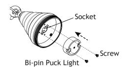
Insert the Bi-pin brass puck light into the socket and secure it in place with the two screws previously removed from the clip.
