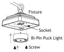
Insert the Bi-Pin brass puck light into the socket and secure with the two screws provided. Tighten with a screw driver.
