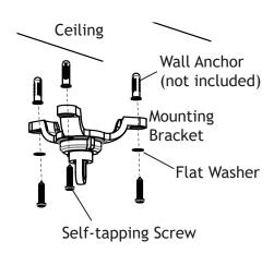
Attach the mounting bracket onto the desired ceiling surface. Secure with the flat washers and self-tapping screws.
