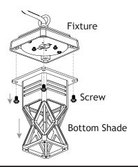
Use a screwdriver to remove the screws from under the fixture. Then take off the bottom shade.
