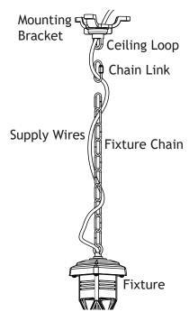
Adjust the fixture chain to the desired length by removing the links if needed. (Note: Pliers are required for this step).
