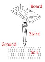
Determine the desired location for mounting the luminaire. Hammer the stake into the ground until the flange of stake is flush to grade. To avoid damage to the stake, place a board on top of stake while hammering.
