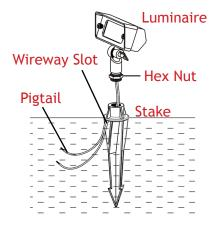
Clear away an area in the ground at the wireway slot on top of the stake. Lay the luminaire pigtail into the wireway slot and screw the fixture on to the stake. Tighten the hex nut on the luminaire against the stake and tighten until snug.
