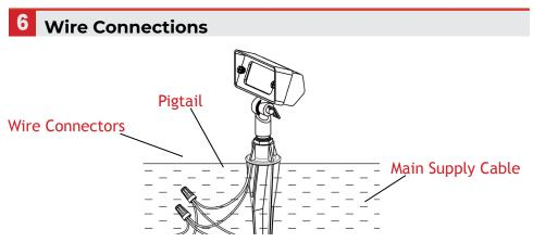
Strip both leads from the luminaire pigtail. Using two wire connectors (sold separately), connect the leads from the luminaire to the main supply cable leads.
