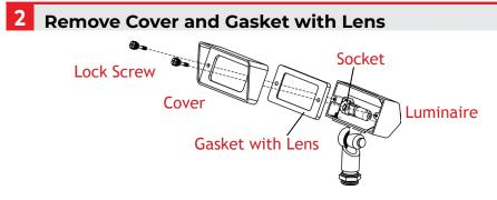
Loosen the lock screws and remove the cover and gasket with the lens from the luminaire to expose the socket.
