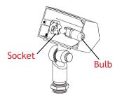
Insert the bulb with correct wattage and type marked on the luminaire label.
