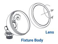
Loosen the lens and remove it from the fixture body by rotating it counter-clockwise.
