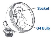
Insert G4 bulb with correct wattage and type marked on fixture label.
