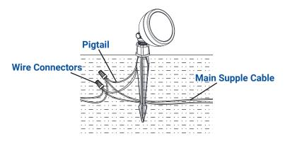
Strip both the leads from the luminaire pigtail. Using two UL listed wire connectors (sold separately), connect the leads from the luminaire to the main supply cable leads.
