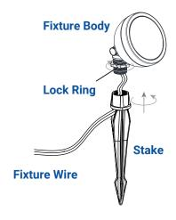
Pass fixture wire through the stake and thread the stake onto the fixture body. Screw the lock ring against the stake and hand tighten until snug.
