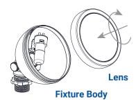
Thread the previously removed lens back onto the fixture body and hand tighten until snug.
