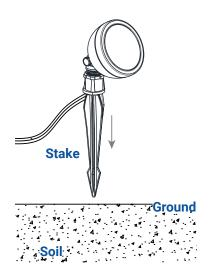
Determine the desired location for mounting the fixture. Insert the stake into the ground until flange of stake is flush to grade.
