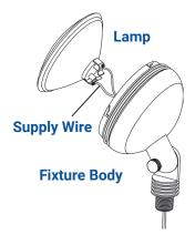
Use a PAR36 lamp (sold separately), with correct wattage and type as marked on luminaire label.
