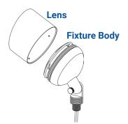
Install the lens to the fixture body by aligning the locking parts on both of them. Be sure to position the lens so when it turns it locks properly into place.
