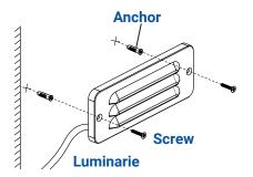
Note: Anchors are required for concrete or brick walls. Hold the luminaire on the wall and mark two points for the anchors using the mounting holes as guides. Then drill the proper holes using the marks. Insert the anchors into the drilled holes.
