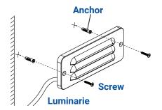
Note: Anchors are required for concrete or brick walls. Hold the luminaire on the wall and mark two points for the anchors using the mounting holes as guides. Then drill the proper holes using the marks. Insert the anchors into the drilled holes.
