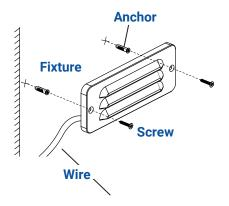
NOTE: Must be mounted with the wire on the bottom. Note: Anchors are required for concrete or brick walls. Hold the fixture on the wall and mark two points for the anchors using the mounting holes as guides. Then drill the proper holes using the marks. Insert the anchors into the drilled holes.
