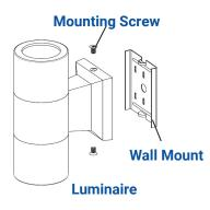
Remove the mounting screws off the top and bottom of the luminaire and remove the luminaire from the wall mount.
