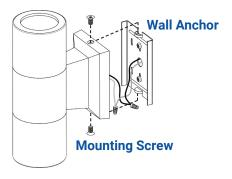
Carefully tuck all the wires into the wall mount. Attach the back of the luminaire over the wall mount. Secure it by threading the mounting screws onto the top and bottom of the luminaire body.
