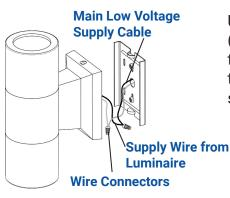
Using two wire connectors (sold separately) connect the supply wires from the fixture to the main low voltage supply cable leads.
