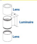
Twist the top and bottom lens to remove them from the luminaire.
