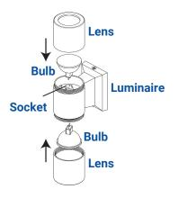
Insert the bulbs (sold separately) with the correct wattage and type marked on the luminaire label.
