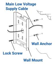
Place the wall mount at the desired location and mark two points on the wall surface for the wall anchors. Remove the wall mount and drill the proper holes on the wall.
