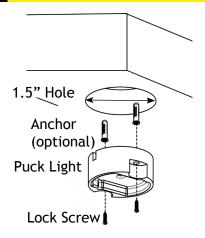
Using a 1.5" core drill bit, drill a hole in the desired flat surface. Attach the puck light into the drilled hole and secure with the lock screws.
