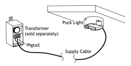
Lay the supply cable out from the transformer. Strip both leads from the luminaire pigtail. Connect the leads from the luminaire supply cable to the transformer (sold separately).
