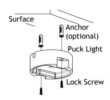
Attach the puck light to the flat surface (under railings, shelves, counters, benches, or any other niche location). Secure with lock screws.
