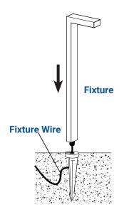
Pass the fixture wire through the center hole of the stake. Thread the fixture on to the stake and hand tighten until snug.
