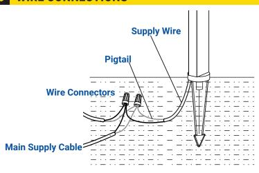
Strip both leads from fixture body. Using two wire connectors (sold separately), connect the leads from the fixture body to main supply cable leads.
