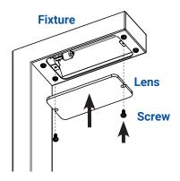
Place the lens back onto the fixture and secure with the previously removed screws. Tighten until snug.
