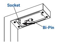
Insert the Bi-Pin with correct wattage and type marked on fixture label and push into place.
