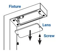
Remove the lens from the fixture by loosening the screws.
