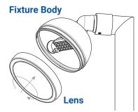
Install the lens back onto the fixture body and hand tighten until snug.
