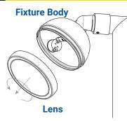
LOOSEN the lens and remove it from the fixture body by rotating it counter-clockwise.
