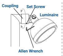
By using the Allen wrench, loosen the set screw at the coupling. Rotate the coupling with luminaire to your desired direction. Tighten the set screw with Allen wrench once your desired direction is achieved.
