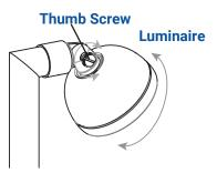
Loosen the thumb screw at the joint. Rotate the luminaire to your desired direction. Tighten the thumb screw once your desired direction is achieved.
