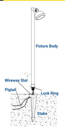
Clear away an area in the ground at the wireway slot on top of the stake. Lay the luminaire pigtail into the wireway slot and screw the fixture body on to the stake. Tighten the lock ring against the stake and hand tighten until snug.
