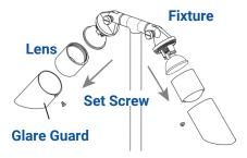
Loosen the set screws and remove the glare guards from the lens. Then remove the lens from the fixture.
