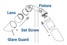
Place the lens over lamps and thread onto fixture. Attach glare guards back onto the lens and secure with set screws.
