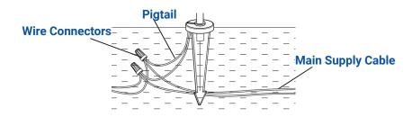
Strip two leads from luminaire pigtail. Using two wire connectors (not provided), connect leads from luminaire to main supply cable leads.
