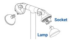
Insert lamp with correct wattage and type marked on fixture label.
