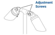
By using screwdrivers, loosen adjustment screws and adjust lamps to your desired angles and then tighten adjustment screws.
