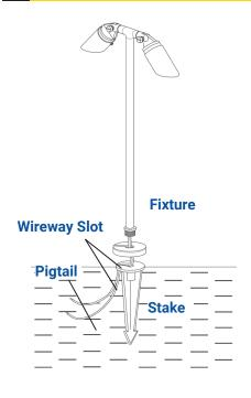
Clear away area in ground at wireway slot in top of stake. Align the wireway slots on base and stake. Lay luminaire pigtail into wireway slots and screw fixture into stake. Tighten until snug to secure base.
