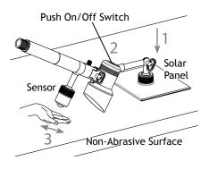
Place the solar light on a nonabrasive surface with the solar panel face down. Press the ON/ OFF switch on the back of the fixture body. Wave your hand in front of the sensor to test the fixture.
