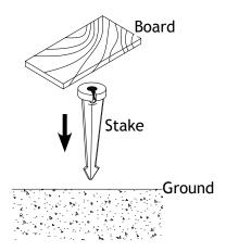
Determine the desired location for mounting the stake mount. Hammer the stake into the ground until flange of stake is flush to grade. To avoid damage to the stake, place a board on top of the stake while hammering.
