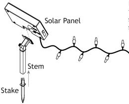
Insert the stem into the back of the solar panel and attach the stake onto the bottom of the stem.
