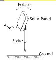
Push the stake into the ground. Rotate the solar panel to the proper direction and lock it into place using the set screw.
