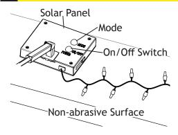
Press the ON/OFF switch on the back of the solar panel while it is face down on a non-abrasive surface.
