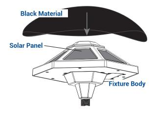
Cover solar panels completely by using black materials. The fixture will light up when the solar panel is covered and turn back off when it is uncovered.
