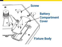
Place the battery compartment cover back onto the fixture body and secure with the previously removed screws.
