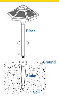
Thread the riser on to the stake and hand tighten until snug.
