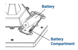
Insert the battery into the battery Compartment.
