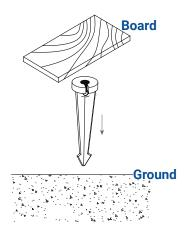
Determine the desired location for mounting the stake mount. Hammer the stake into the ground until flange of stake is flush to grade. To avoid damage to the stake, place a board on top of the stake while hammering.
