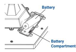
Insert the battery into the battery Compartment.
