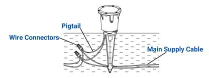
Strip both leads from the luminaire pigtail. Using two wire connectors (sold separately), connect leads from luminaire to the main supply cable.
