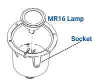
Insert lamp with correct wattage and type marked on fixture label.
