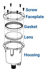
Unlock the screws and remove the faceplate, gasket, and lens from the housing.
