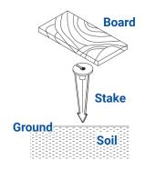
Determine the desired location for mounting the fixture. Hammer the stake into the ground until flange of stake is flush to grade. To avoid damage to the stake, place a board on top of the stake while hammering.
