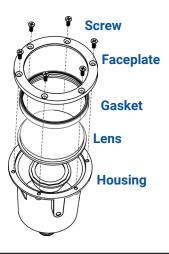
Place the lens, gasket and faceplate back onto the housing. Secure them with screws previously removed. Hand tighten until snug, then use a screwdriver to secure them in a star
