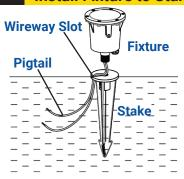
Clear away an area in the ground at the wireway slot on top of the stake. Lay the luminaire pigtail into the wireway slot and screw the fixture onto the stake. Tighten until snug.
