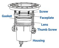
Loosen the thumb screws and slide the housing down to the end of the bars. Unscrew the screws and remove the faceplate, gasket, and lens from the housing.
