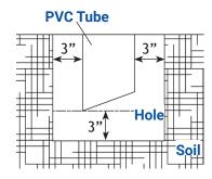
Dig a hole in the ground making sure there is approximately 3 inches of room on all sides surrounding the PVC tube for pea gravel or sand.
