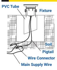
Place the fixture onto the PVC Tube. Pass the luminaire pigtail through the PVC tube.
