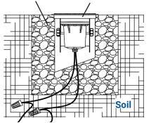
Install the PVC tube with fixture in the hole and fill the extra space with pea gravel or sand for proper water drainage.
