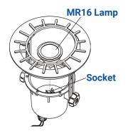
Insert the lamp with the correct wattage and type marked on the fixture label
