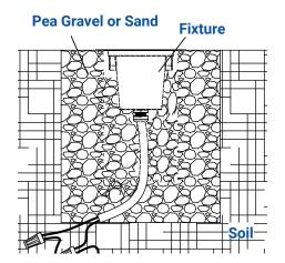
Install the fixture in the hole and fill the hole with pea gravel or sand.
